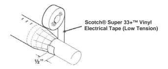
7.6 Bundle mold's notched ends evenly around cable, maintaining cable centering. Starting 1/2" (12 mm) on cable jacket, apply 1 half-lapped layer of Scotch® Super 33+™ Vinyl Electrical Tape over notches. (Figure 12)
