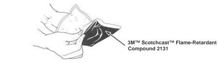
8.2 Firmly grasp each flat side of the closed mixing pouch near the center barrier; at the same time, pull sides of barrier apart and roll sides of thumbs through barrier. Break the barrier all the way across to the side seals. (Figure 13)
