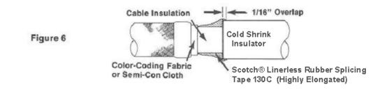
4.4 Apply highly elongated Scotch<sup>®</sup> Linerless Rubber Splicing Tape 130C to cable insulation at ends of cold shrink insulators, forming tapers to insulators Extend tapers from cable color-coding fabric and/or semi-conducting cloth to 1/16" (2 mm) onto insulators. (Figure 6)
