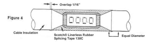
4.1 Smoothly fill in connector area with half-lapped, highly elongated Scotch® Tape 130C; *BUILD UP TO DIAMETER OF CABLE INSULATION,* overlapping 1/16" (2 mm) beyond pencils. (Figure 4)
