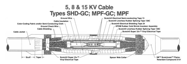
NOTE: On large 15kV cables, additional Scotch® Tape 130C, Scotch® Tape13 and Scotch® Tape 24 may be required.
