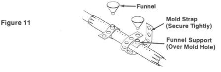
7.5 Position Funnel Supports over mold holes and secure tightly with Mold Straps. (Figure 11)
